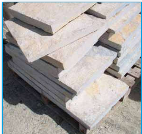
Newly prepared Purbeck stone paving
